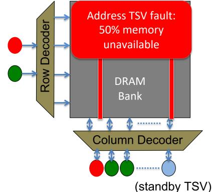
Data vs Address TSV Faults Using CRC-32+BIST
