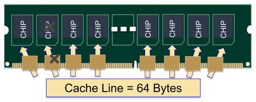
ChipKill: Mitigate Large Failures (Whole Chip)
