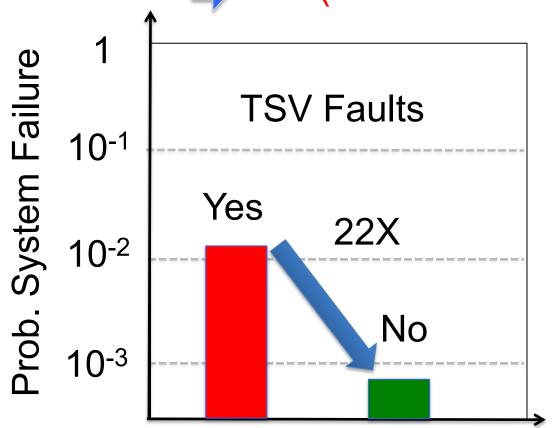
Efficient Techniques to Mitigate TSV Faults
