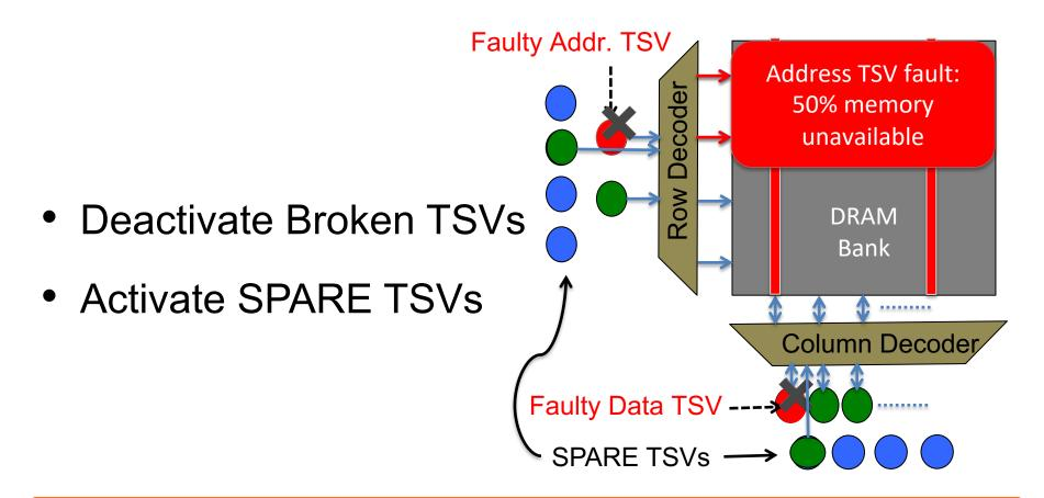
Deactivation of Faulty TSVs and Activation of Spare TSVs is performed at design time
