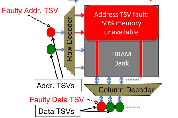
TSVs can cause failures at multiple granularities
