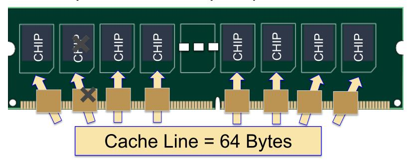
ChipKill: Mitigate Large Failures (Whole Chip)
