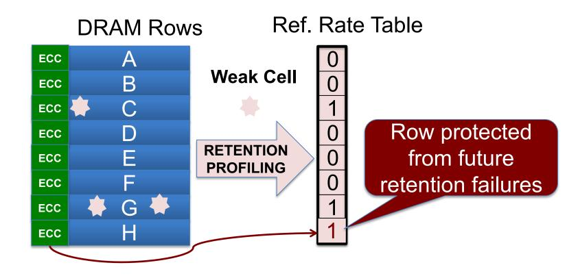
Insight: Avoid forming Active VRT Pool  $\rightarrow$  Upgrade on ECC error Observation: Rate of VRT >> Rate of soft error (50x-2500x)
