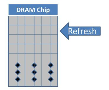
Retention Time: The time for which cell/memory retains data
