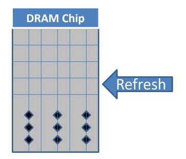
Retention Time: The time for which cell/memory retains data
