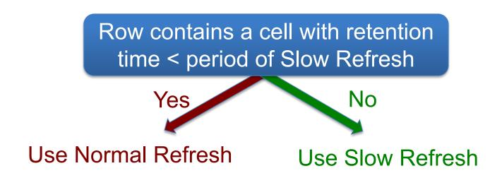
Retention time of cells vary significantly: most cells >> 64ms
