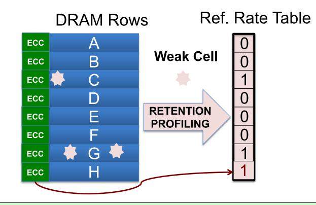
Insight: Avoid forming Active VRT Pool  $\rightarrow$  Upgrade on ECC error Observation: Rate of VRT >> Rate of soft error (50x-2500x)
