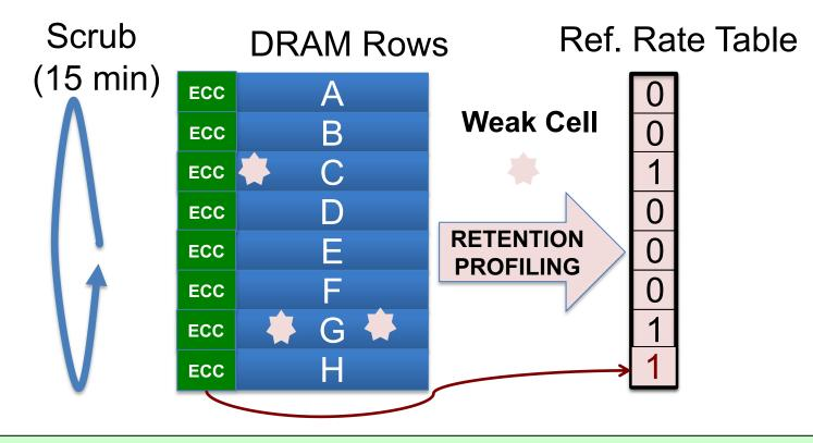
Insight: Avoid forming Active VRT Pool  $\rightarrow$  Upgrade on ECC error Observation: Rate of VRT >> Rate of soft error (50x-2500x)
