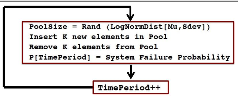
Input: Mu,Sdev, for the logn of Active-VRT pool Input: K, rate of discovering new VRT cells
